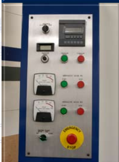
Digital line speed & thickness displays
