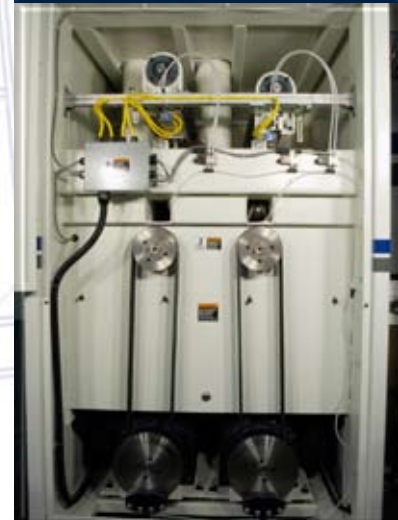
Individual TEFC drive motors with disc brake & pneumatic caliper
