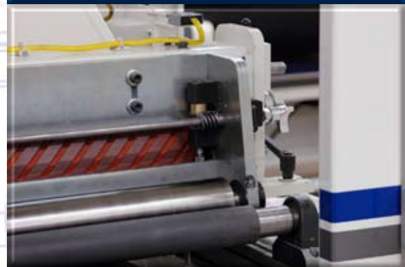
Adjustable platen with helical worm gear design
