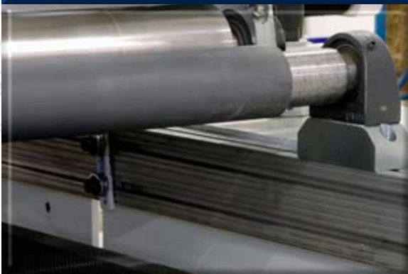
Heavy duty spring-loaded pinch rollers
