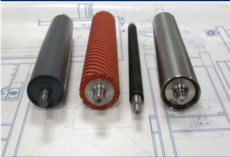
Large diameter rollers and drum for precision operations
