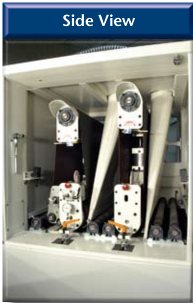
Two-head model with drum and combination head
