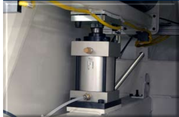
Large bore pneumatic cylinder
