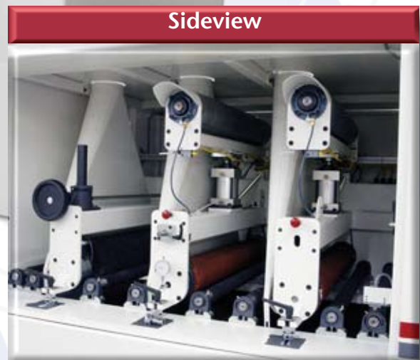
Three head configuration with two abrasive belts and one brush head.
