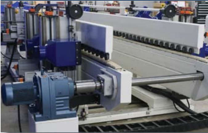
Dual chain assemblies and (2) upper hold down beams.
