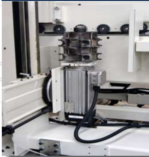
Vertical spindle shaper with stacked tooling to reduce setup.
