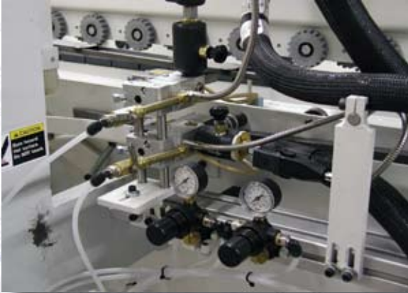
Electro/pneumatic controlled glue dispensing heads with adjustable flow controls.
