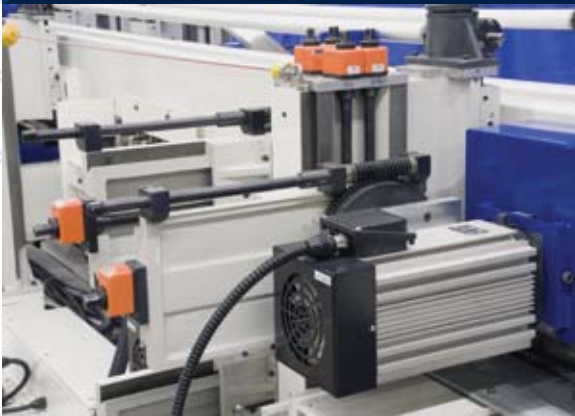
Double cast iron columns with machined dovetail slides and individual dial indicators.
