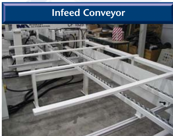
Infeed wheel conveyor with overhead rack for staging build-down, scribe and no-drip sticks.
