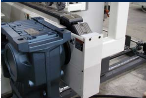
AC drive motor coupled directly to drive sprocket.
