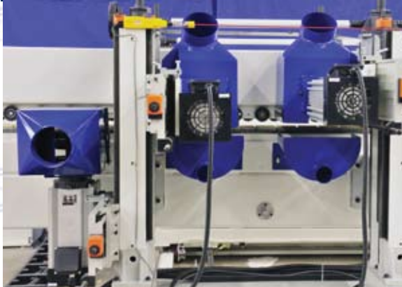
Horizontal and vertical spindle shapers on dovetail slides.
