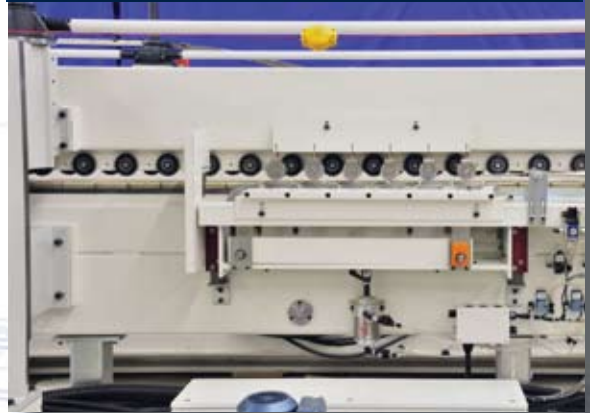
Spring-loaded stick clamping system aligns and holds sticks to the edges of the core.
