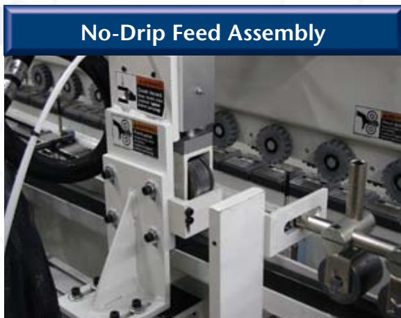
Optional No-Drip Stick System with pneumatic clamping.
