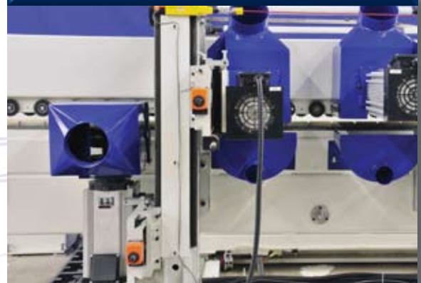
Double cast iron column with sizing and shaping units.
