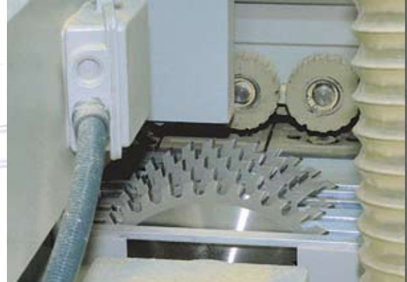
Cutter head assembly with sizing saws engineered to specific customer requirements.
