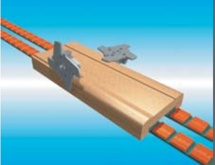
Sticks are directed to top and/or bottom of panel and clamped until bond is completed.
